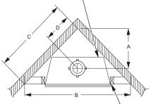
3/4" Clearance Not Required at Nailing Flanges
